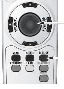
\_PRESENTATION POINTER button Move the pointer on the screen with this button.
